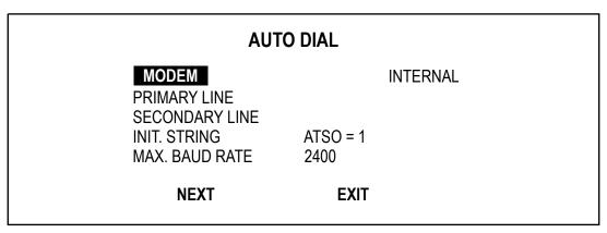
To get to the Modem Selection screen, highlight MODEM and press SELECT. The following screen will come up showing that the modem is disabled.
